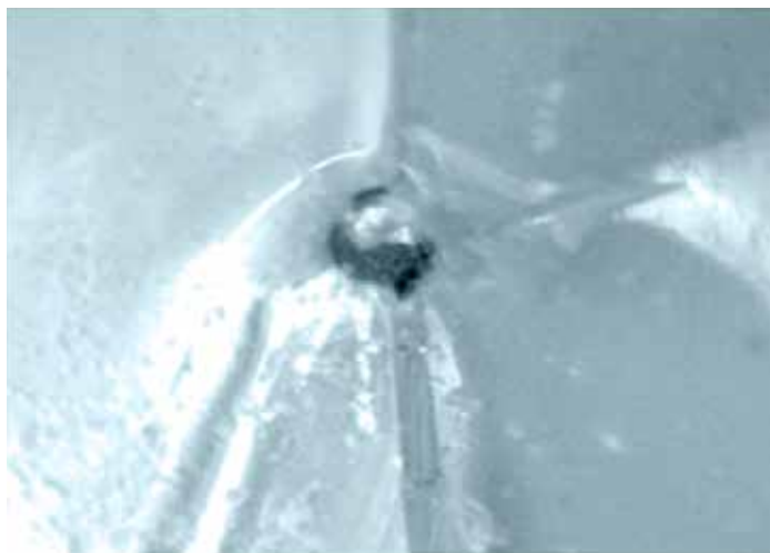
Nickel sulfide inclusion — .006219"
