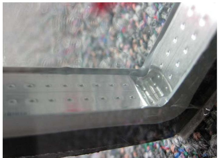
Viracon has performed testing on insulating glass units that have PIB visible in the vision area and these units have performed comparably to units that may not have PIB completely covering the aluminum spacer. Due to Viracon's specification and design of the
