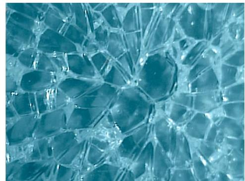
FIGURE 2: FULLY TEMPERED GLASS, NICKEL SULFIDE BREAK PATTERN
