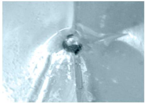
FIGURE 1: MAGNIFIED NICKEL SULFIDE INCLUSION .006219"
